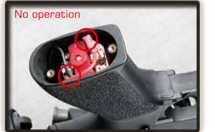
No operation Check the wire set contact on the motor.
