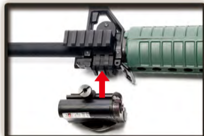
G-12-001 Install the visible laser.
