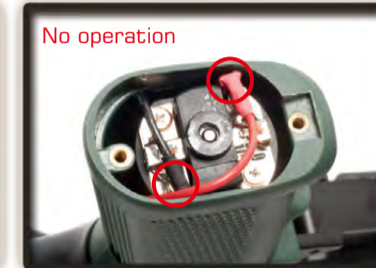
Check and make sure the motor wires are connected to the motor.
