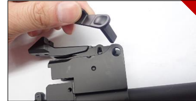
Turn the box to the other side then Install Handguard Fixer
