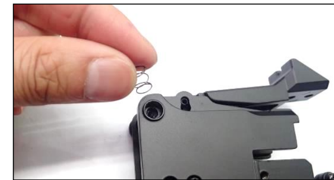
Turn the box to the other side then Install Handguard Fixer
