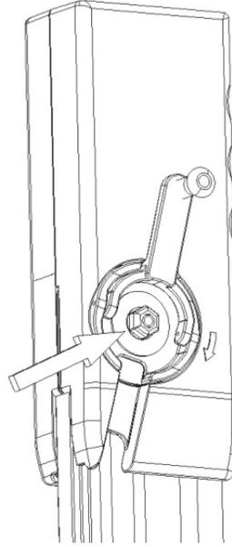
Some magazines have stiffer springs than industry standard, and might require the adjustment of the clutch nut. If your magazines are not getting fully loaded, locate the clutch nut on your M12 Sidewinder, and using a 10mm wrench, rotate it clockwise 1/8 turn, and attempt to load the magazine again. Repeat this step until the M12 loads your magazine completely.
