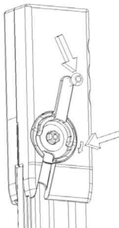
Hold the M12 Sidewinder in a vertical position with the loader on top, and rotate the crank arm in a clockwise manner. Once the magazine is full, the clutch will engage.
