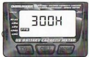
Servo test Frequency Setting Mode Servo Test Frequency Setting: 50Hz, 60Hz, 100Hz, 125Hz, 200Hz, 250Hz, 300Hz
