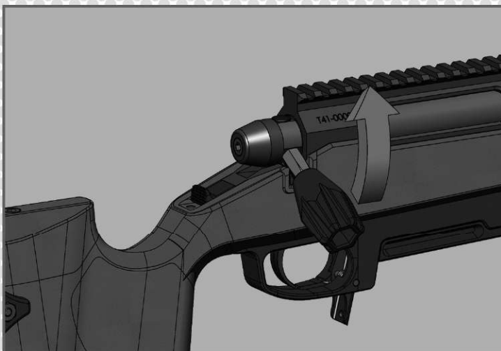
Lift up the bolt handle (make sure the bolt is not already loaded to avoid double feeding).
