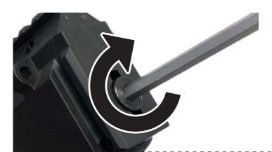
When installing or reinserting the spring guide, the locating tabs on the guide are inserted and the 12 and 6 o'clock positions. The guide should then be rotated through 90 degrees and the tabs should seat in the internal recesses at the 3 and 9 o'clock positions.
