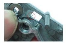
3. Assembly and lock the screws, please make sure that the spring cannot be shown outside the Cut-Off Lever.
