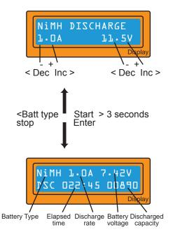
The discharge current is shown on the left and the voltage of the pack on the right. The discharge current ranges from 0.1A to 1.0A and the final voltage ranges from 0.1V to 25.0V). You can alter the parameters by pressing **Start/Enter**. Once the correct values have been input, press **Start/Enter** again to store the values. To start the process, hold **Start/Enter** for 3 seconds.
