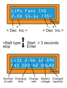
You can set up the charging current and the voltage of the battery pack which is being charged. Press **Start/Enter** to bring up the voltage confirmation screen. If the voltage and current parameters are correct, press **Start/Enter** again to start the charging process.
