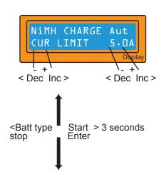
This program charges the battery using the charge current set by the user. In 'Aut' mode, you must set the charge current limit to prevent the charger feeding too much current into the battery, which could cause damage. In 'Man' mode, the battery will be charged with the charge current set by the user. You can change the mode by pressing **INC** and **DEC** button simultaneously when the current field is blinking.
