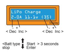
On this screen the top line displays the battery type and the second line shows the charge current and the voltage of the battery pack.
