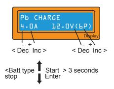
The charge current is shown on the left and the nominal voltage of the battery on the right. The charge current ranges from 0.1A to 6.0A and the voltage should be matched with the battery being charged. To start the charge process, hold **Start/Enter** for 3 seconds.
