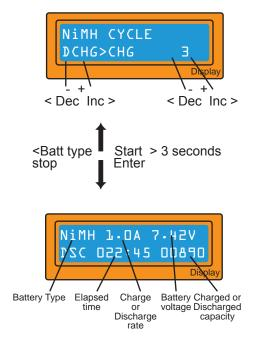
On this screen you can alter the cycle sequence on the left and the number of cycles on the right. The 'CYCLE' mode can be used for balancing, refreshing and 'breaking-in' the battery. A time delay will occur after each charge and discharge process to allow the battery adequate time to cool down before being subjected to the next process. This delay is set on the 'User Settings' menu.
