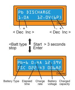
The discharge current is shown on the left and voltage of the battery pack on the right. The discharge current ranges from 0.1A to 1.0A. You can alter the parameters by pressing **Start/Enter**. Once the correct values have been input, press **Start/Enter** again to store the values. To start the discharging process, hold **Start/Enter** for 3 seconds.
