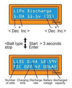
The discharge current (shown on the left side of the screen) should not exceed 1C and the final voltage on the right should not be under the voltage level that is recommended by the battery manufacturer to avoid deep discharging. To start the discharge process, hold **Start/ Enter** key for 3 seconds.
