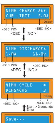
Here you can set up the charge current for the manual charge mode, or the current limit for the automatic charge mode. Each mode can be switched by pressing **INC** and **DEC** at the same time when the current field is blinking.
