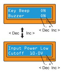
The beep sounds every time a button is pressed to confirm your action. Beeps or melodies may be sounded at various times during operation to alert the user of different mode changes. You can turn these sounds on and off.
