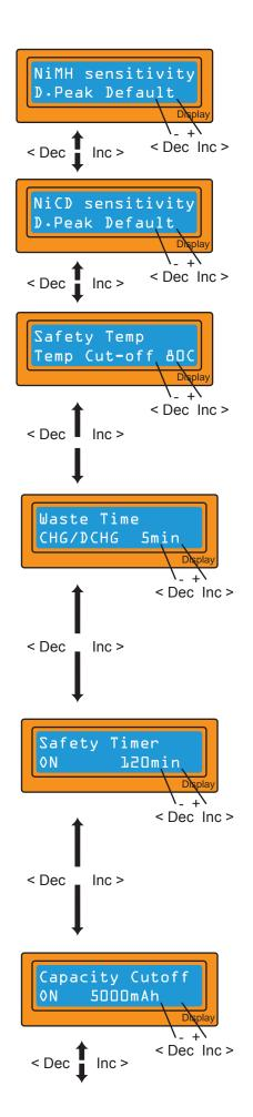
This shows the trigger voltage for automatic charge termination of NiMH and NiCd battery. The effective value ranges from 5 to 20mV per cell. If the trigger voltage is set higher, there is a danger of overcharging the battery; if it is set lower, there is a possibility of premature termination. Please refer to the technical specifications of the battery. (NiCd default: 12mV, NiMH default: 7mV)
