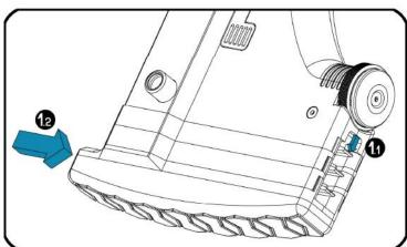
While pressing the tab backwards, push the buttplate down to remove it. Using the end buttplate spacer (SRS214) is mandatory for pull bolt, and using at least one buttplate spacer is highly recommended. For push bolt SRS, make sure the bolt is in foward position before to remove the buttplate.
