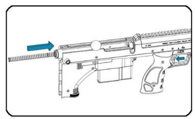
While the trigger is pulled back, slide the bolt head, the cylinder assembly, the piston & spring inside the receiver.
