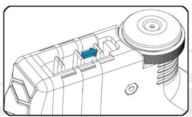
Make sure the tab is in the locked position (toward the receiver)
