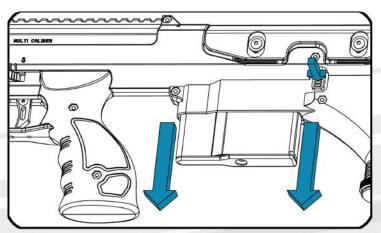
4 You can also remove the magazine using the left side magazine release button.
