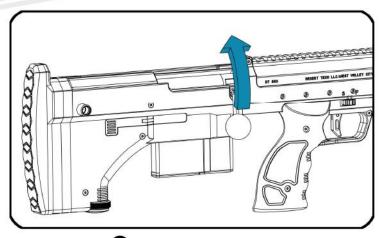
Pull up the bolt handle. A Make sure that the bolt is not already armed to avoid double feed.
