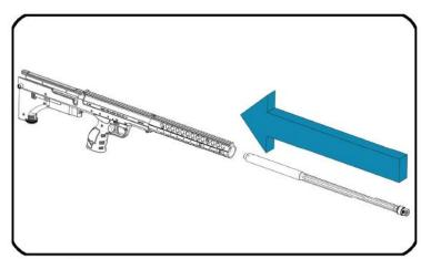
Gently insert the barrel inside the receiver.
