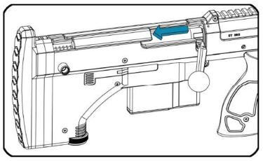
8 Insert the dust cover into the ejection window, then slide backward.
