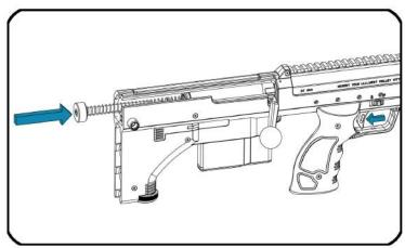
3 While the trigger is still pulled back, insert the spring guide inside the spring. Push on the end of the spring guide, compressing the spring inside the end of the receiver.
