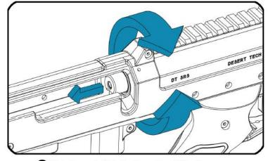
② Rotate and slide the barrel until the hopup fits onto the BB-tube.
