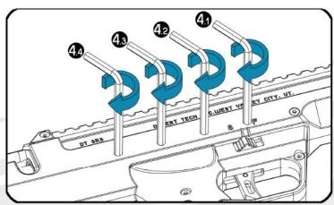
4 Secure the barrel by tightening the 4 barrel screws, from muzzle to bolt side (and reverse order for removal).
