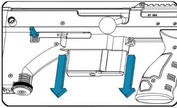
3 To remove the magazine, pull the magazine down after depressing the right side magazine release button.
