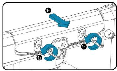
Loosen the two M5x6 screws.
