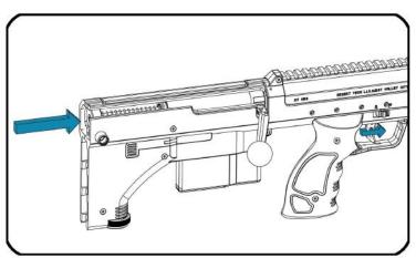
4 After pushing the spring guide inside the end of the receiver, release the trigger and push it forward. Keep forward pressure on the trigger in order to lock the spring guide inside the receiver.
