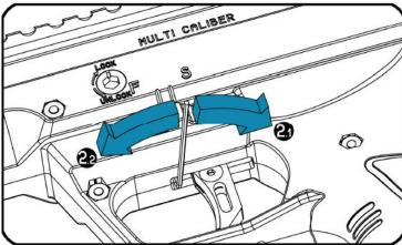
To adjust the trigger pull weight, tighten the M3x12 trigger screw to increase the pull weight. 200sen the M3x12 trigger screw to decrease the trigger pull weight.
