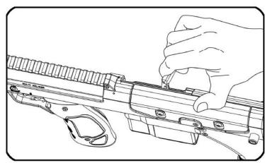
3 It is recommended that you pull the bolt by grabbing the bolt handle as close to the cyclinder as possible (to reduce friction and ease priming movement).
