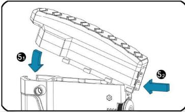
While the trigger is still pushed front, slide buttplate into place starting at the bottom and sliding up.
