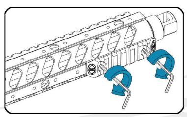
2 Secure the rail using two M4x7 screws from the screw set bag.
