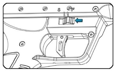
1 Slide the safety button (right or left) to «S» position to engage the safety.
