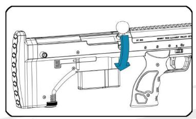
5 Lock down the bolt handle to lock the bolt.
