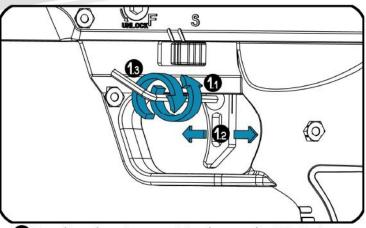
To adjust the trigger position, loosen the M3x6 trigger screw. Slide the trigger forward or back to the desired position. Tighten the M3x6 trigger screw to lock the position of the trigger.
