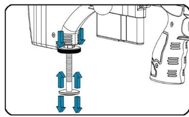
2 For fast adjustment, push up or down on the monopod foot, while holding the monopod knob.
